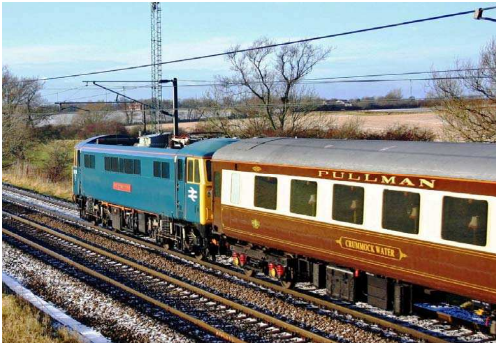
Above – Trailing at the rear was Class 86 No.86101 (Note the pantograph is lowered).
